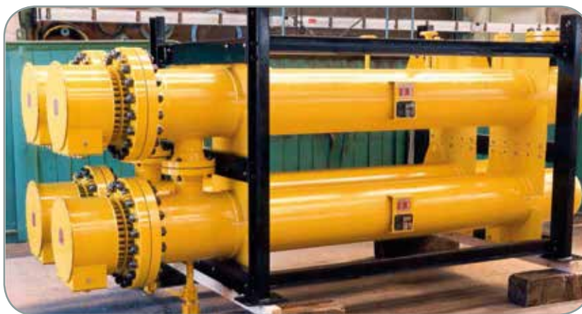
Circulation heater for heavy fuel in power plant
